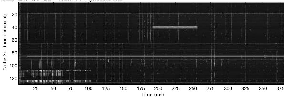
**Figure 4: Sample memorygram collected over an idle period of 400ms. The X axis corresponds to time, while the Y axis corresponds to different cache sets. The sample shown has a temporal resolution of 250 s and monitors a total of 128 cache sets. The intensity of each pixel illustrates the access latency of the particular cache set, with black representing low latency and white representing a higher latency.**
