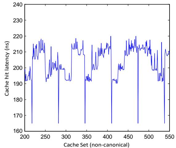
**Figure 7: L3 cache hit times show a 3-level graduation (Haswell i7-4960HQ).**
