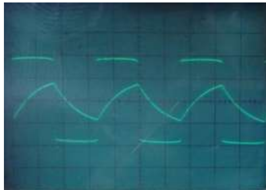
Figure 10. Output waveform with almost equal and fixed duty cycles ( T_{ON} = T_{OFF} ). Scale: X-axis 2 \mu\text{s}/\text{div} and Y-axis 1 \text{ V}/\text{div} .
