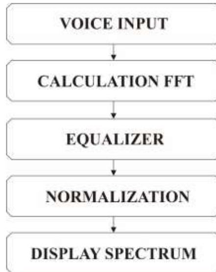
**Figure 2.** Diagram of the Audio Spectrum Analyzer
